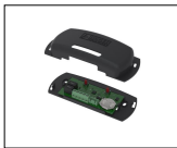
B71/PBX/RTCC Real Time Clock Calendar device for Powerbox Inverters.
