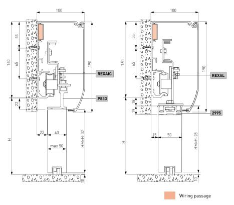
Unless otherwise specified, all measurements are expressed in millimetres (mm). The REX automation wall fixing measurements are illustrated in the diagram, considering that the door wing profiles are not of our production.
