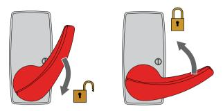
In the event of maintenance, malfunctioning or emergency, lower the lock release lever LOKSBM (if installed) and move the door wings manually into the open position.
