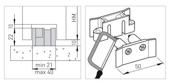
The measurements of the code  $\ensuremath{\mathsf{OKP369}}$  floor guide for glass door wings are indicated in the diagram.
