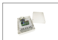
B71/PBX24/BOX/115 Hybrid inverter, "Network Assisted" version, for powering the automation. Also provides a battery-charger function thanks to the connection to the solar panels or mains supply for powering the 24V DC brushless digital controllers with a mains voltage of 115V AC.
